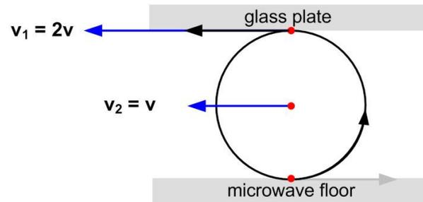
Roller motion relative to microwave floor (center moving).
